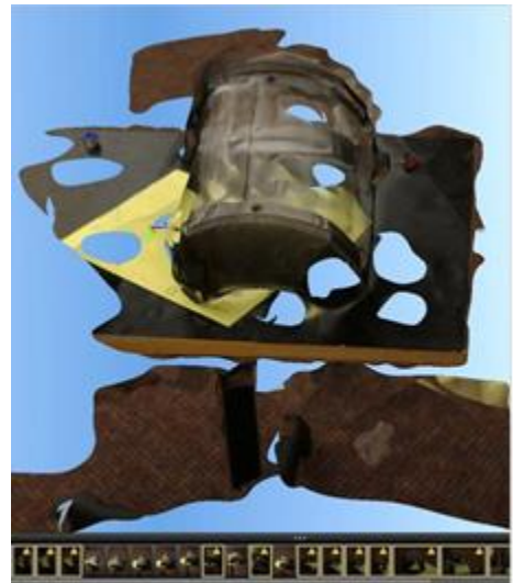
123D Catch had trouble with this clear, shiny, and uniformly colored object.
