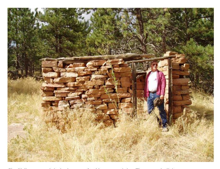
Clay Volkmann stands in the doorway of a old quarryman's hut. These were the living quarters for the quarrymen and were constructed of rejected flagstone pieces, including the roof. The walls were double-rows of stones (offset to cut the wind) and had two windows. Wooden beams supported the roof and sawed wood was used in door and window frames.
